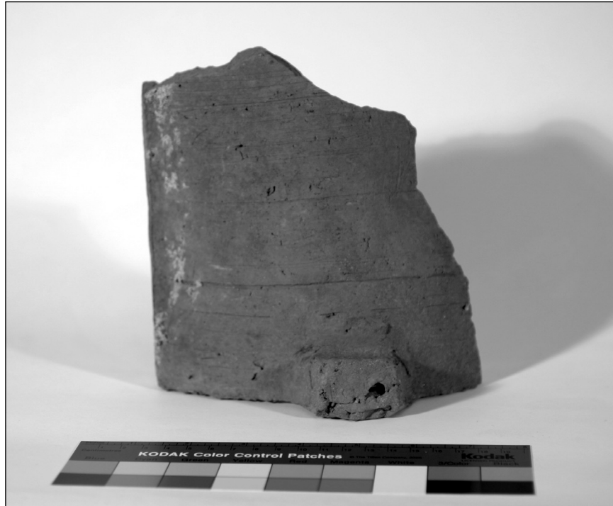
Figure 2. Terracotta roofing tile produced by Frederick Petersen in Salt Lake City, Utah.
